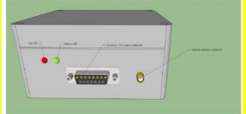
GPS box Sizes: 115x90x55mm Weight: 340g + pipe clamps 110g
