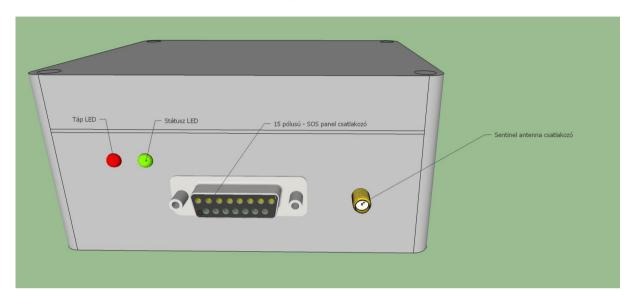
Pic. No. 1.: **GPS box** Sizes: 115x90x55mm Weight: 340g + pipe clamps 110g
